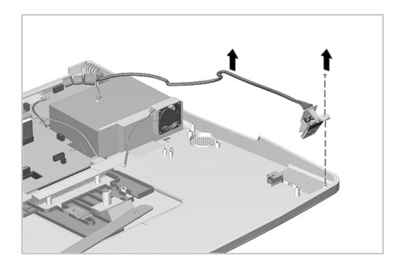
Figure 7-30. Removing the IrDA Board
